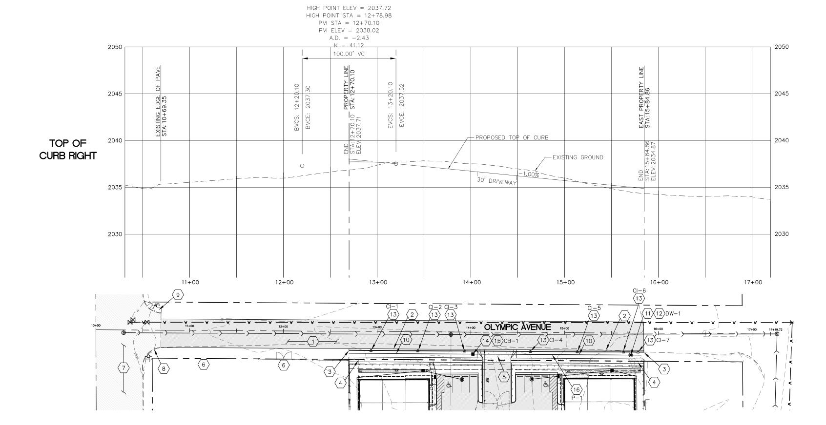
$\langle 2 \rangle$ INSTALL CONCRETE CURB AND GUTTER PER CITY OF SPOKANE STD. PLAN F-106
